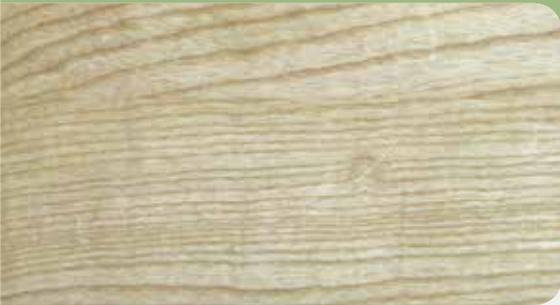
European Ash sapwood is typically white and turns to yellow when exposed to light. The wood has a medium to coarse texture is hard and heavy with very good strength properties. Our European Ash weighs approximately 675kg/m<sup>3</sup>.
